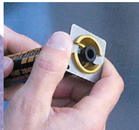
RMS Aft Closure Wrench part #91295 Actual wrench configuration may vary from photo shown.
